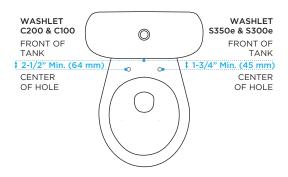
Minimum requirement for front face of tank to the center of mounting holes: C100 & C200: 2-1/2 inches (64 mm) S350e & S300e: 1-3/4 inches (45 mm)
